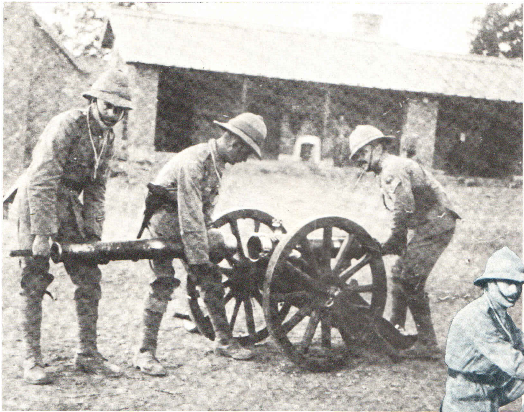
A mountain gun is dismantled before being loaded on to its special mule carriage.
